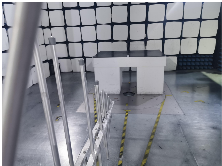
Radiation Emission Test Setup (30MHz to 1GHz)
