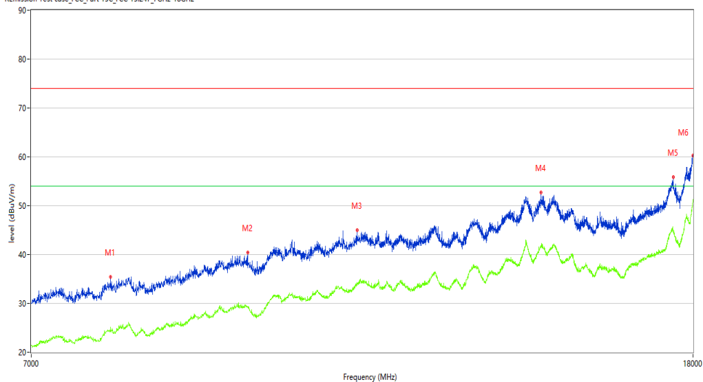
R Emission Test case_FCC_Part 15C_FCC 15.247_7GHz-18GHz
