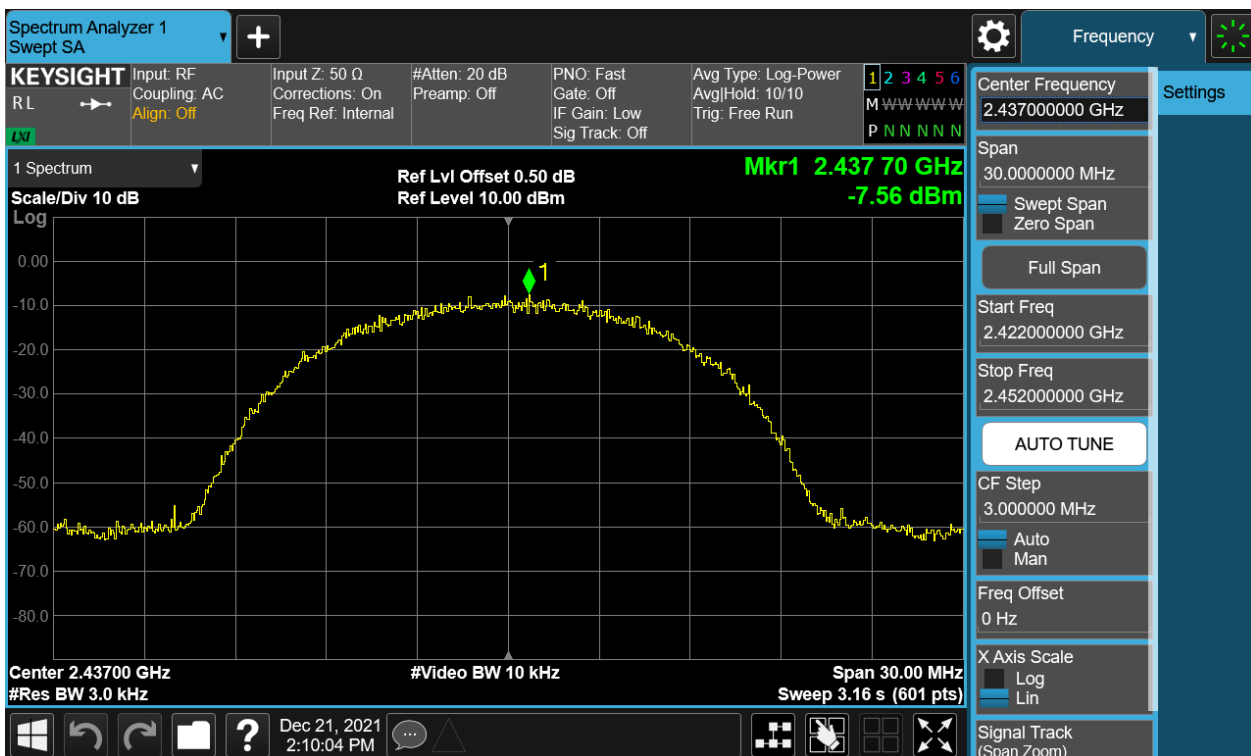
Figure 11: Power Spectral Density, 802.11b, 2437MHz
