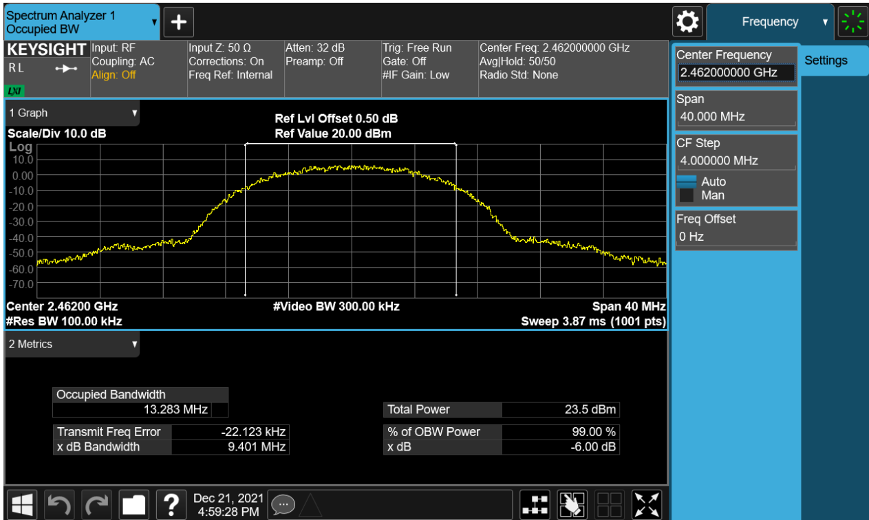
Figure 3: 6dB Bandwidth and 99% Bandwidth, 802.11b, 2462MHz
