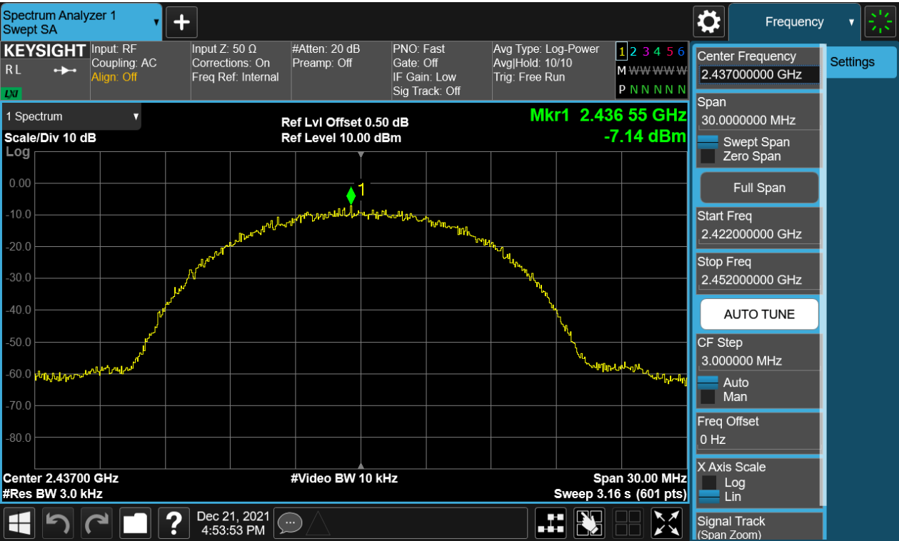
Figure 11: Power Spectral Density, 802.11b, 2437MHz
