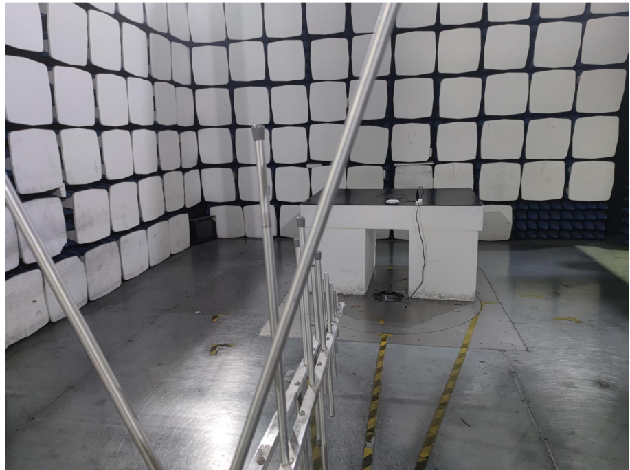
Radiation Emission Test Setup (30MHz to 1GHz)
