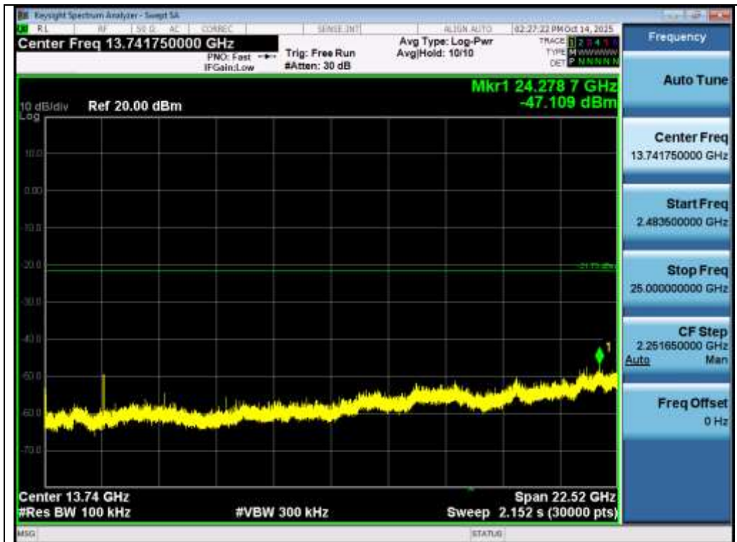
Test_Graph_BR_ANT1_2402_1Mbps_Higher Band Emissions
