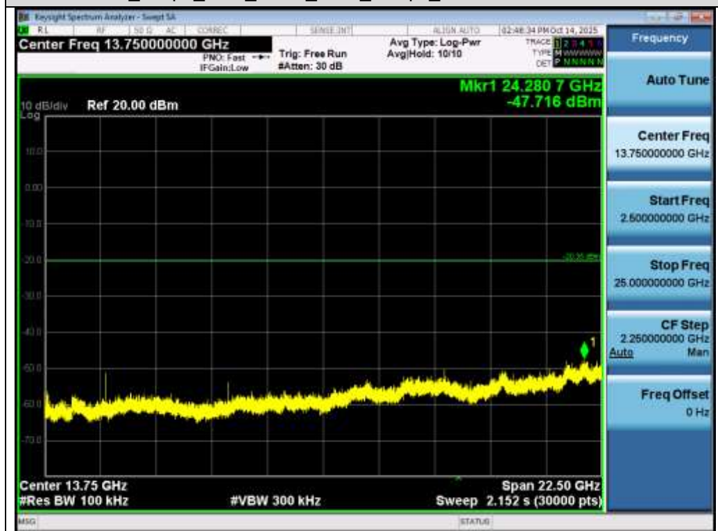
Test_Graph_EDR_ANT1_2480_2Mbps_Higher Band Emissions
