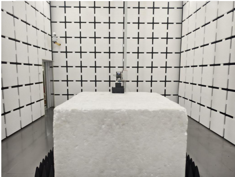
Spurious Radiation Emissions Test (> 1G)
