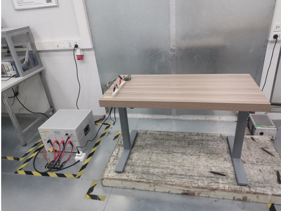
Photo of Conducted Emission Measurement
