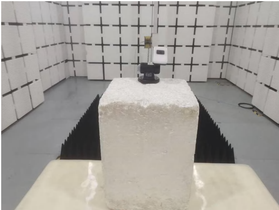
Photograph 2: Set-up for Radiated Spurious Emission, 1GHz - 18GHz
