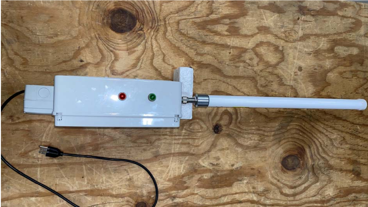
HIFIS Side View with Annunciator LEDs
