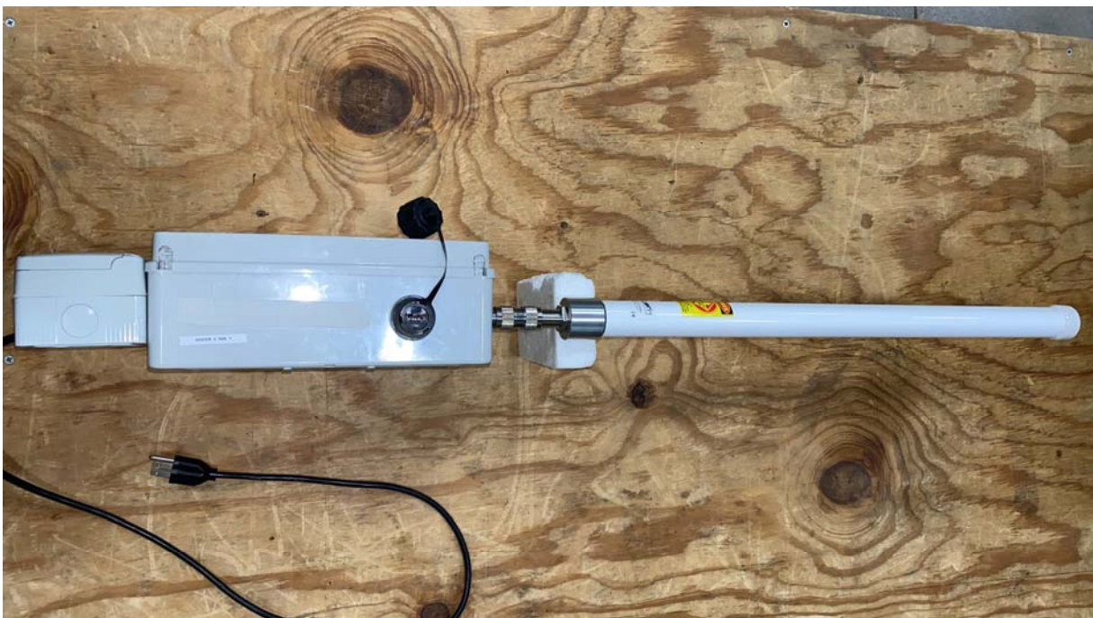
HIFIS Side View with USB Service Port
