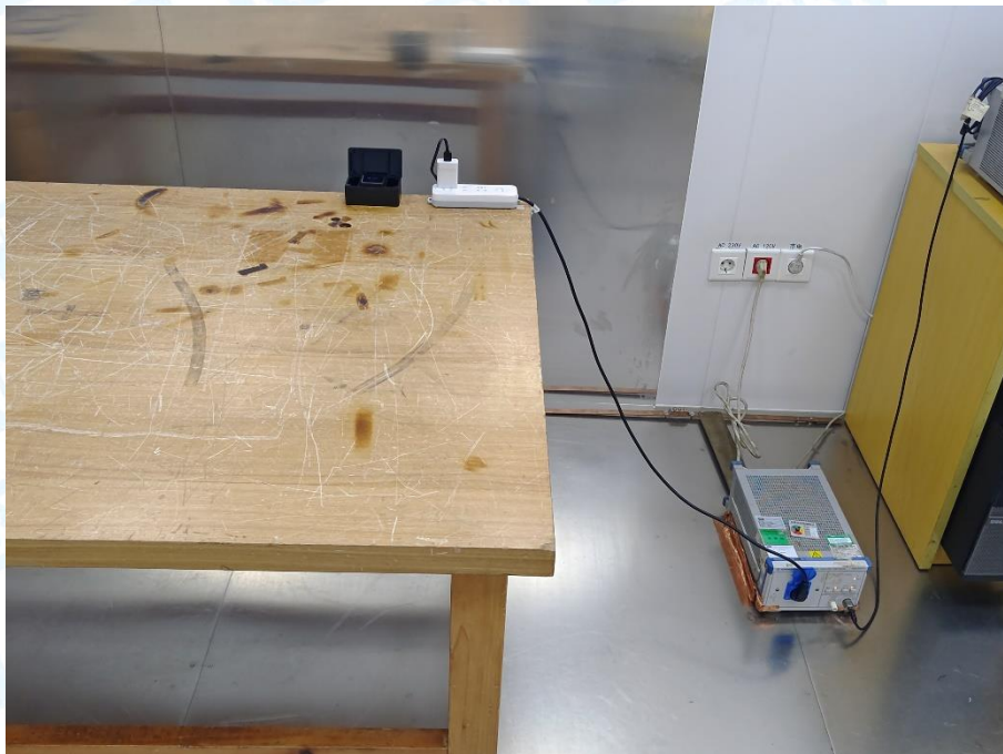
Photo of Setup for Conducted Emission
