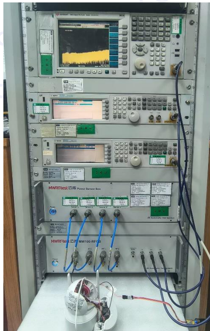
Photo of Setup for Conducted Measurements
