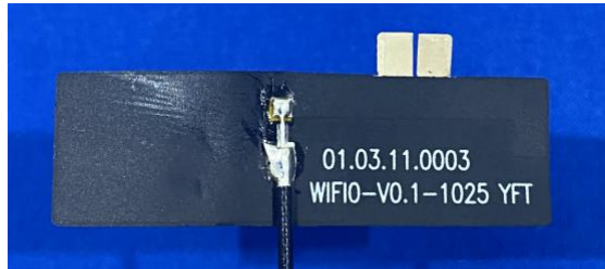
Photo 9: Internal View for BT&WIFI0 ANT
