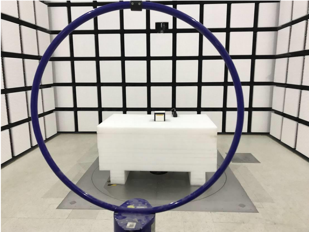
Radiated Emissions 9K-30M View - Perpendicular
