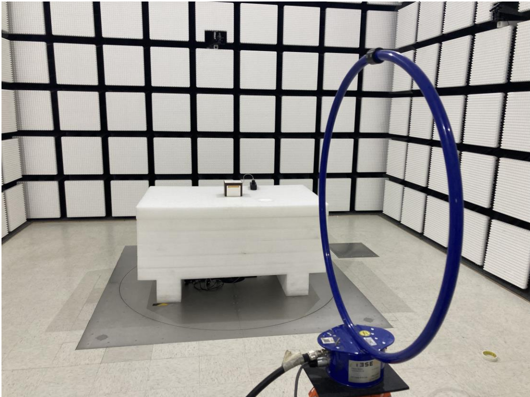
Radiated Emissions 9K-30M View - Perpendicular
