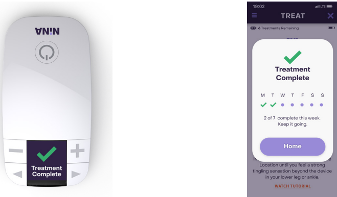
Figure 20. When treatment is complete, a green check mark with the text Treatment Complete will appear.
