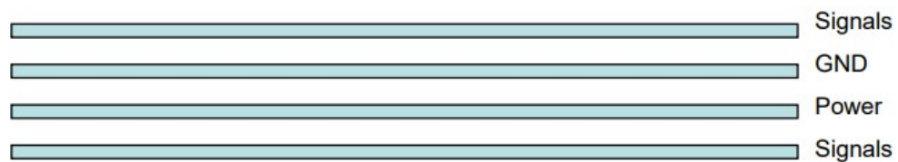
Figure 9: Typical 4-layer PCB construction
