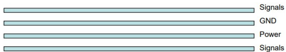
Figure 9: Typical 4-layer PCB construction
