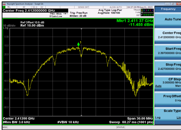
Power spectral density-802.11b ,2462MHz,Ant0
