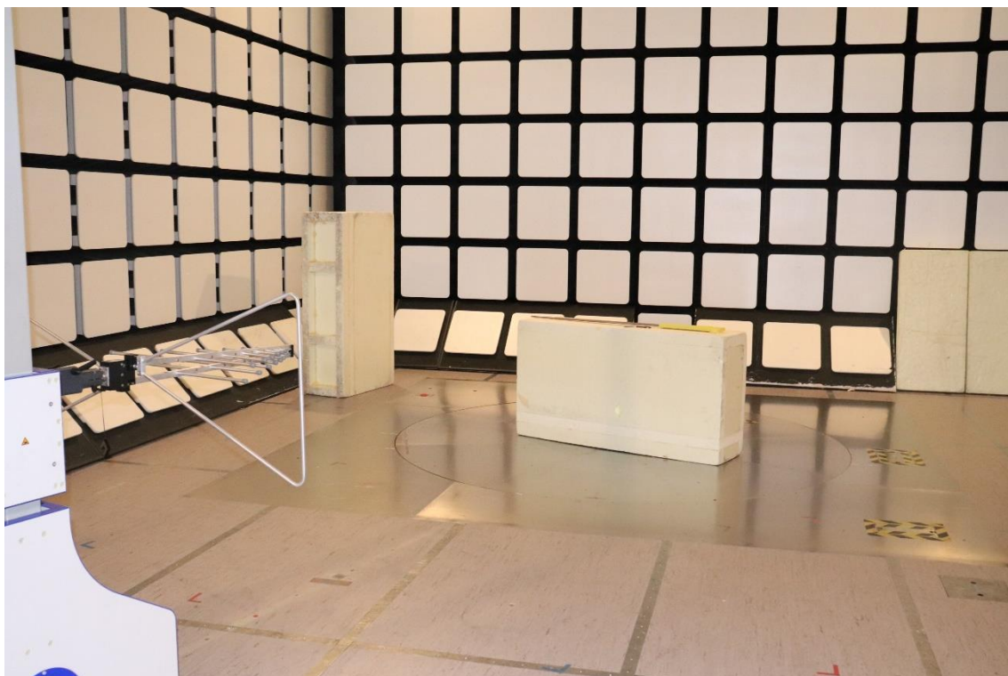
Photograph 3. Radiated emissions 30 - 1000 MHz
