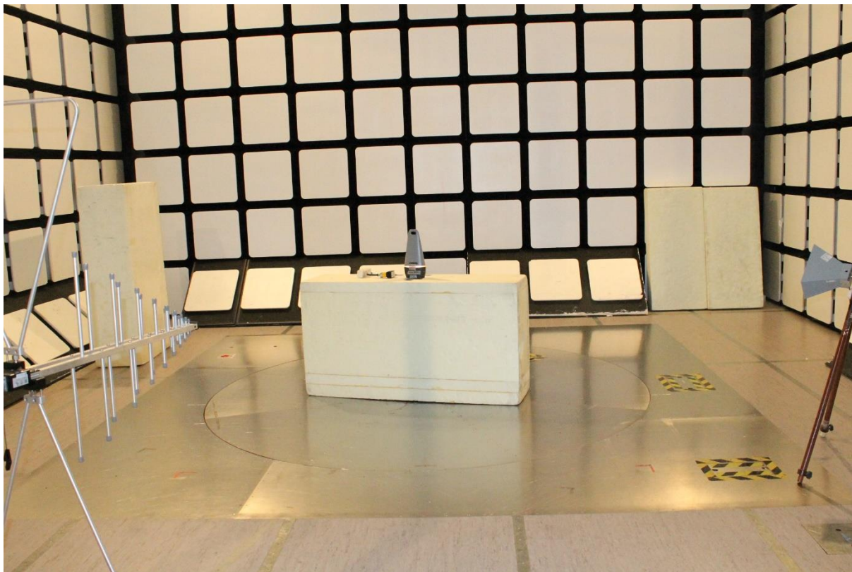
Photograph 1: Radiated spurious emissions setup 30 MHz – 1000 MHz
