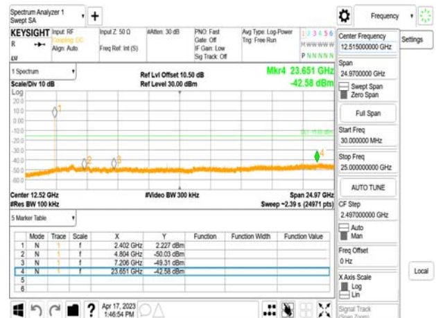
Spurious Emission_BLE 1M_MidCH20-2442MHz
