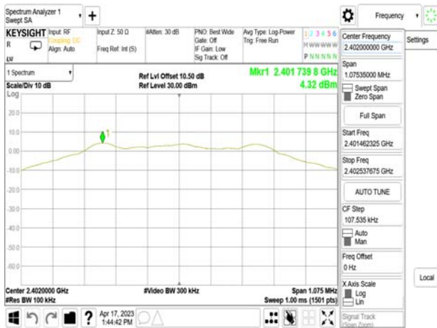
Reference Level_BLE 1M_MidCH20-2442MHz
