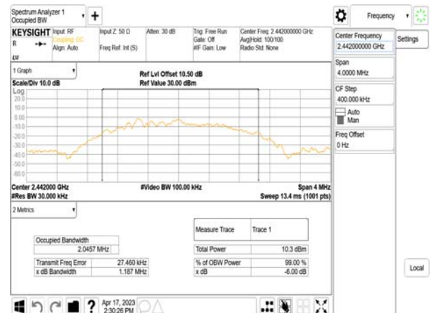
IC OBW_BLE 2M_HighCH39-2480MHz
