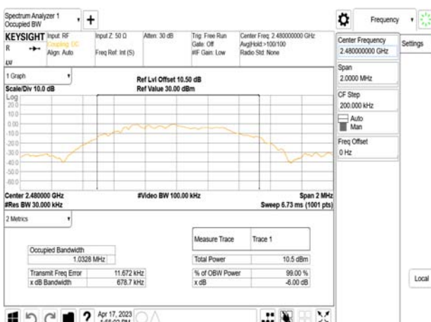
IC OBW_BLE 1M_HighCH39-2480MHz
