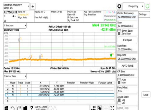
Spurious Emission_BLE 1M_MidCH20-2442MHz
