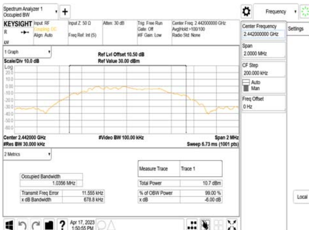
IC OBW_BLE 1M_HighCH39-2480MHz
