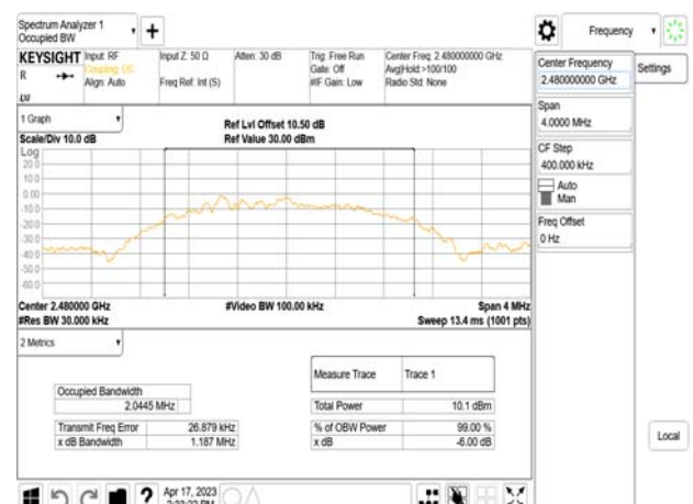
IC OBW_BLE 2M_HighCH39-2480MHz
