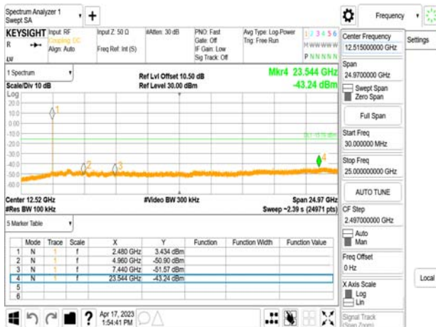
Spurious Emission_BLE 2M_LowCH00-2402MHz
