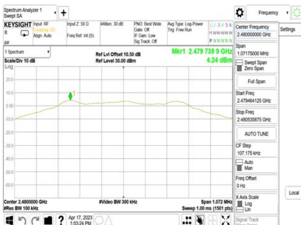
Reference Level_BLE 1M_HighCH39-2480MHz
