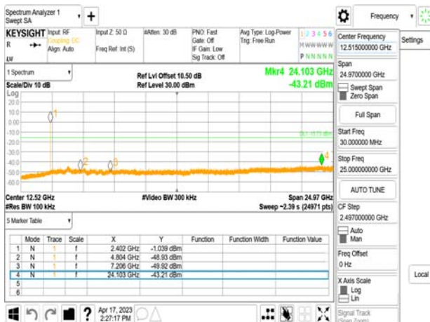
Spurious Emission_BLE 2M_MidCH20-2442MHz
