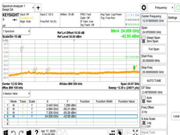
Spurious Emission_BLE 2M_MidCH20-2442MHz
