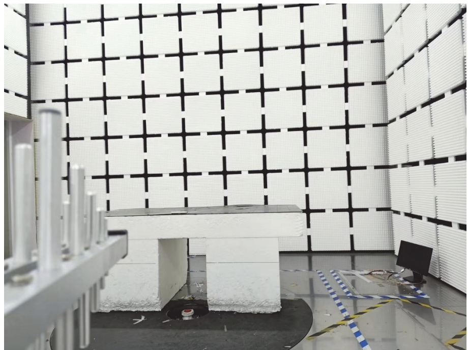
Radiation Emission Test Setup (30MHz to 1GHz)
