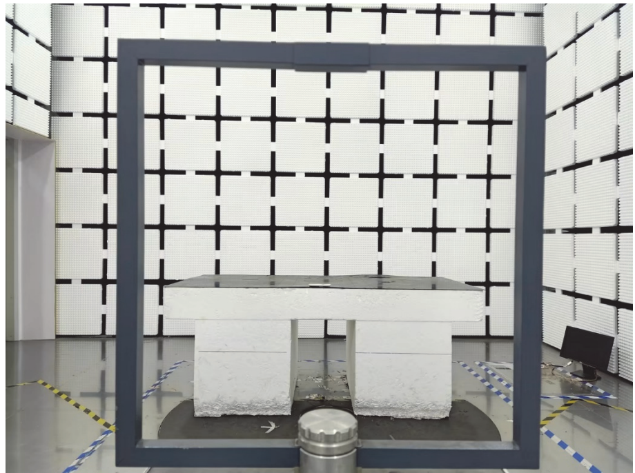
Radiation Emission Test Setup (Below 30MHz)
