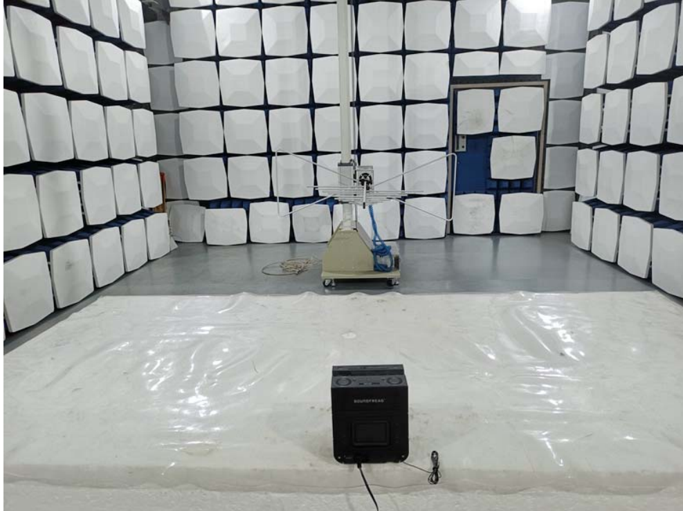
Radiated Emission Test Setup:
