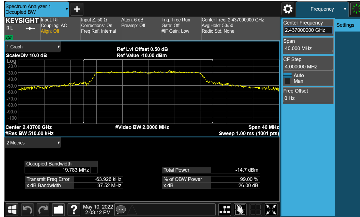
Figure 13: 99% Bandwidth, 802.11g, 2437MHz
