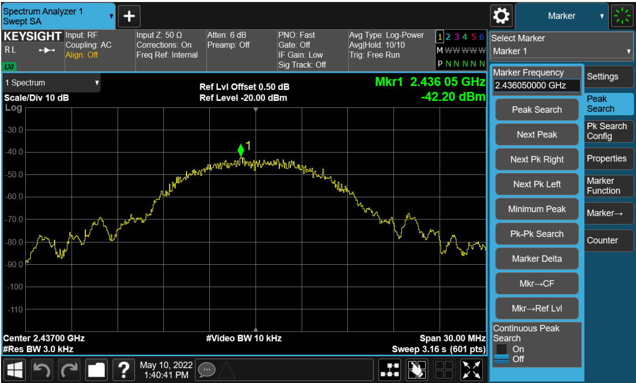
Figure 22: Power Spectral Density, 802.11b, 2437MHz
