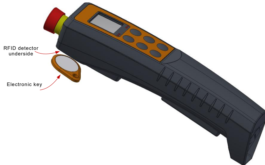
Figure 16: Radio-controlled handheld transmitter RE 6900 user legitimization
