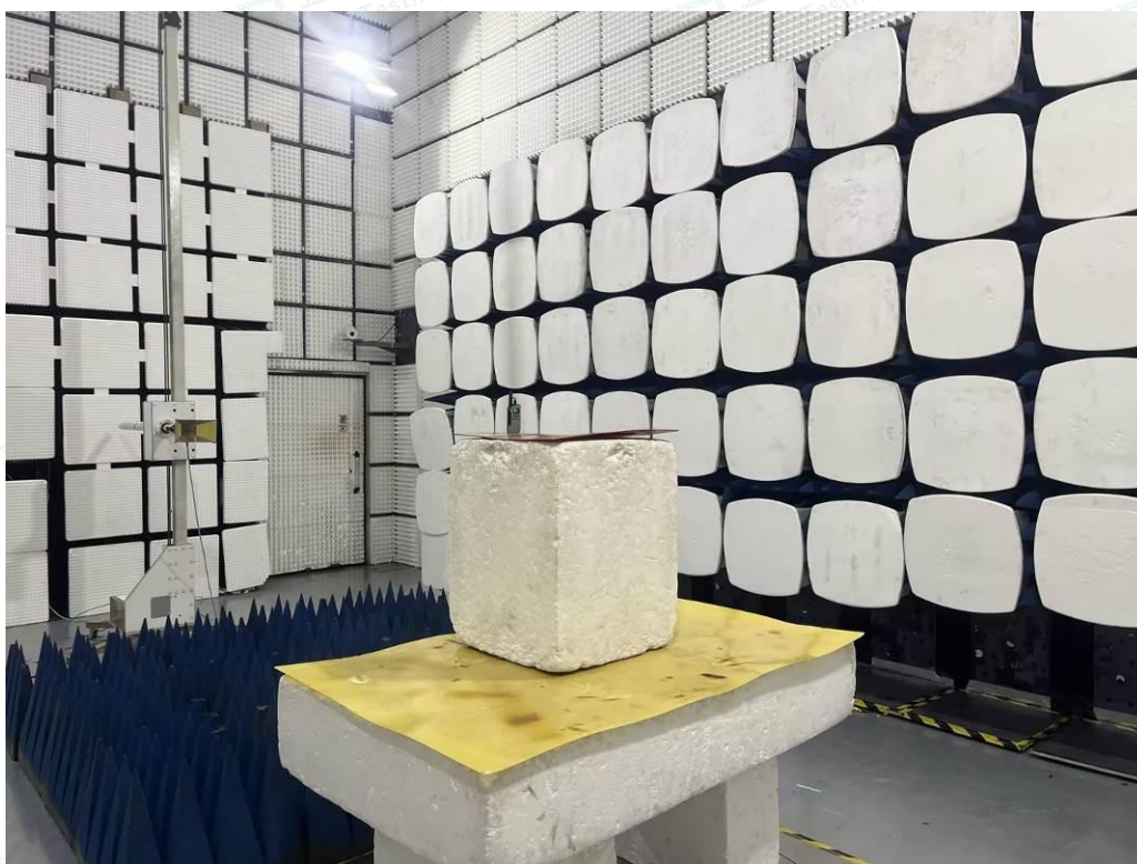
Radiated Emissions Measurement (Above 1GHz)
