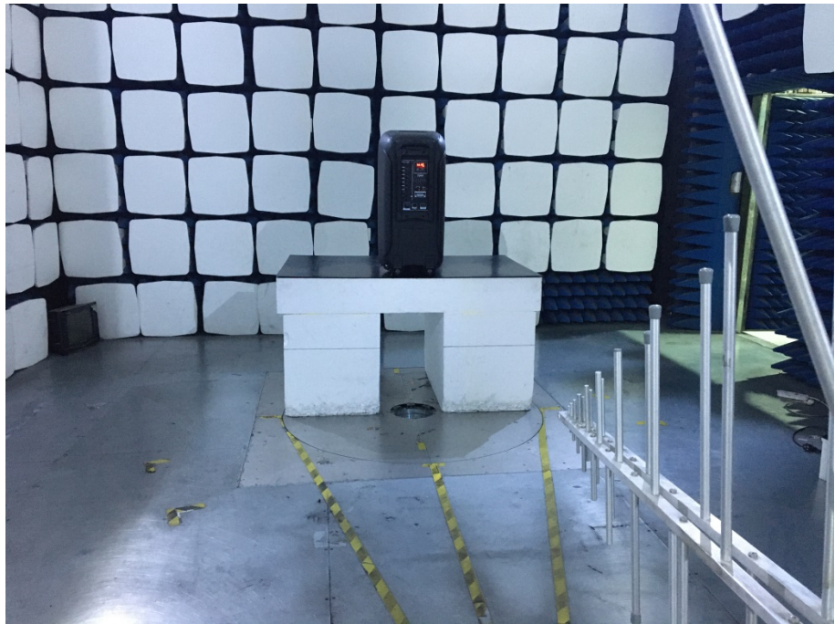
Radiation Emission Test Setup (30MHz to 1GHz)
