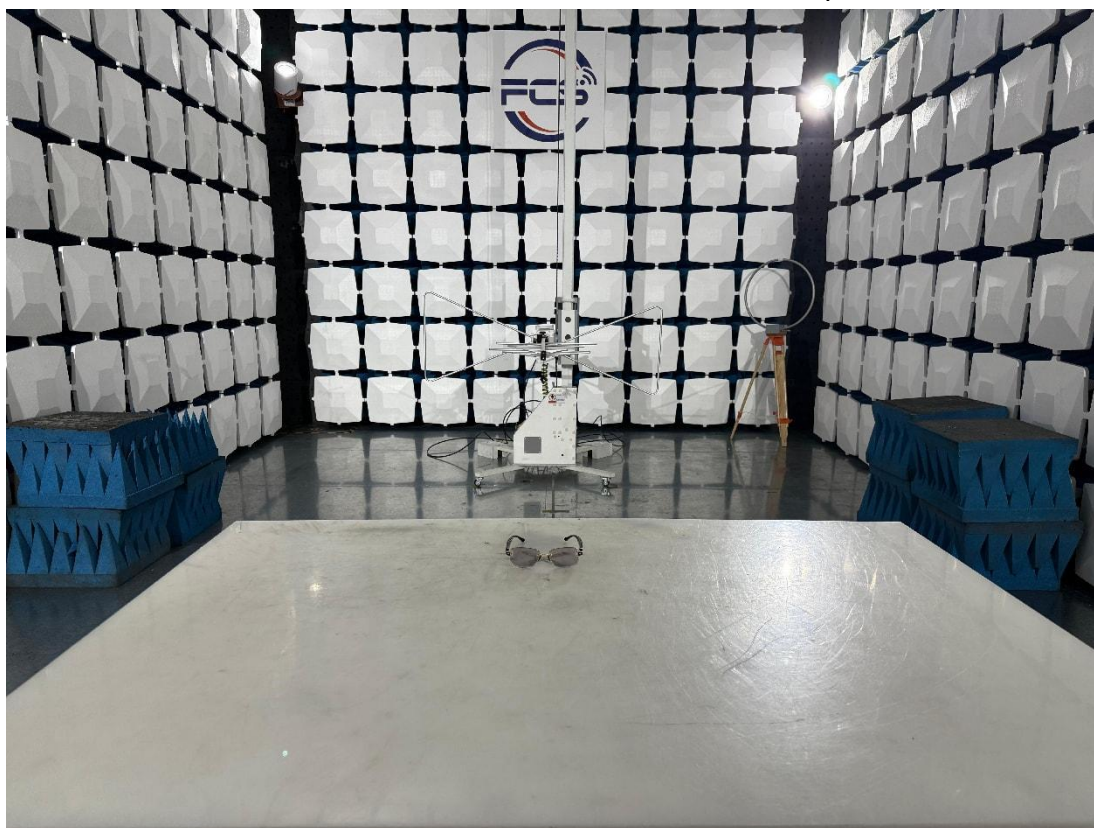
Above 1GHz for radiated emission test setup
