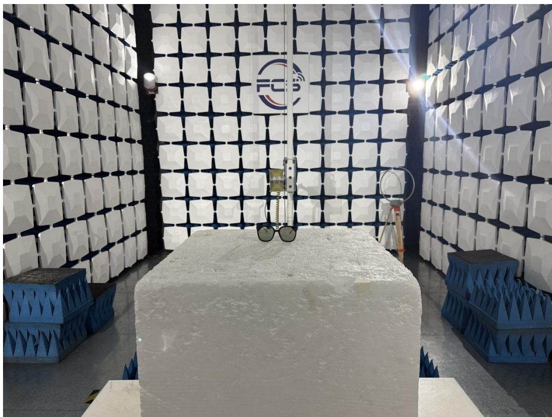
Above 1GHz for radiated emission test setup
