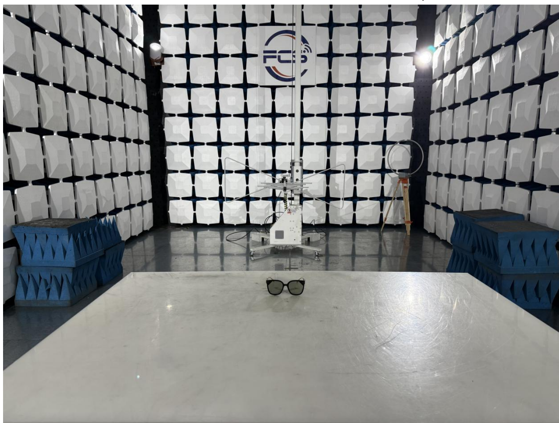
Above 1GHz for radiated emission test setup
