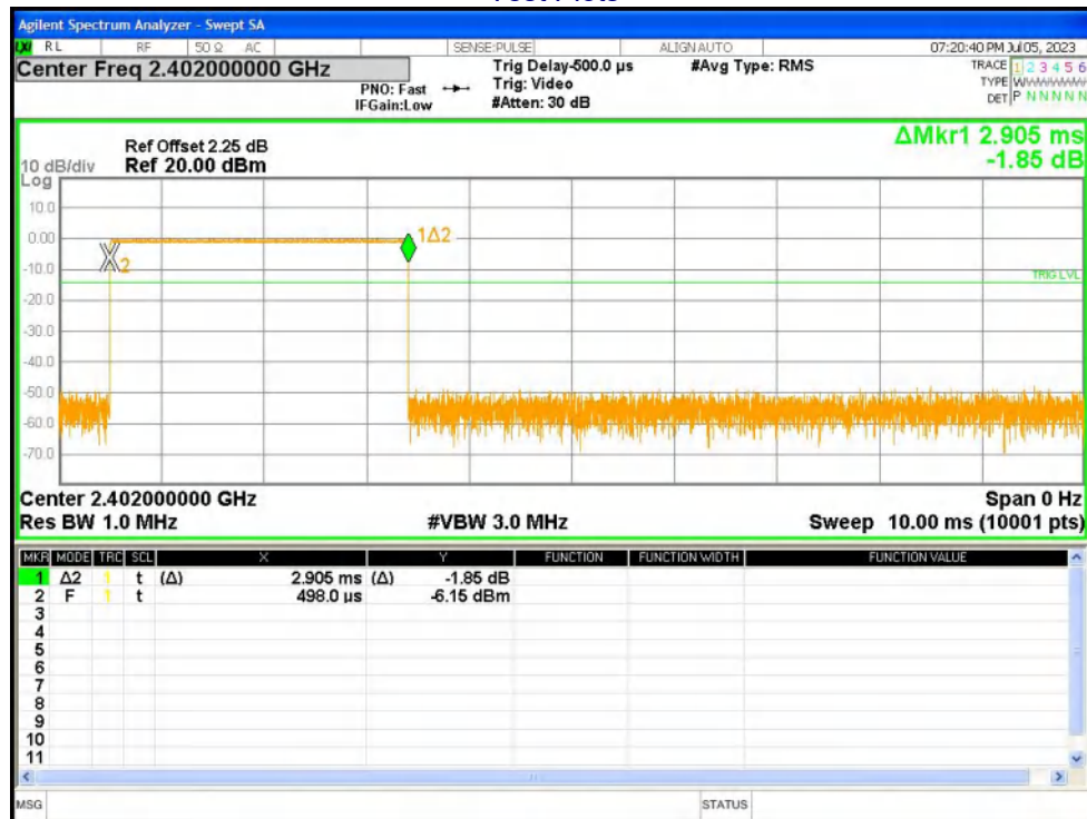
Dwell NVNT 1-DH5 2402MHz Ant1 One Burst
