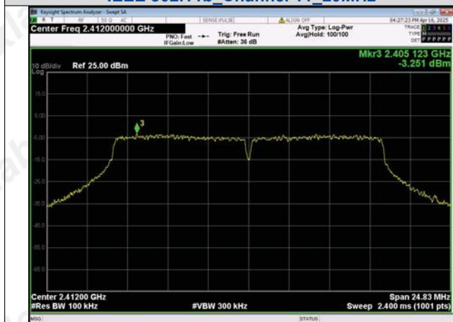
In-Band Reference Level IEEE 802.11g_Channel 1_20MHz
