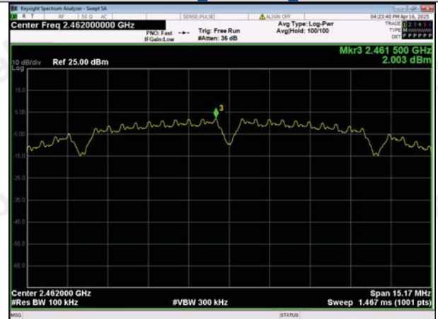
In-Band Reference Level IEEE 802.11b_Channel 11_20MHz
