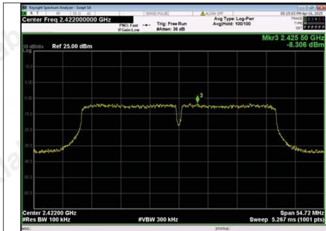
In-Band Reference Level IEEE 802.11n_Channel 3_40MHz
