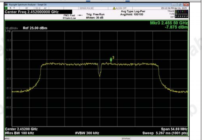
In-Band Reference Level IEEE 802.11n_Channel 9_40MHz
