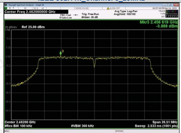
In-Band Reference Level IEEE 802.11n_Channel 11_20MHz
