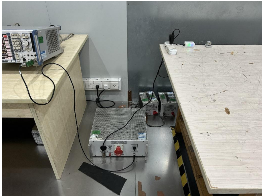
Conducted Emission Test Setup
