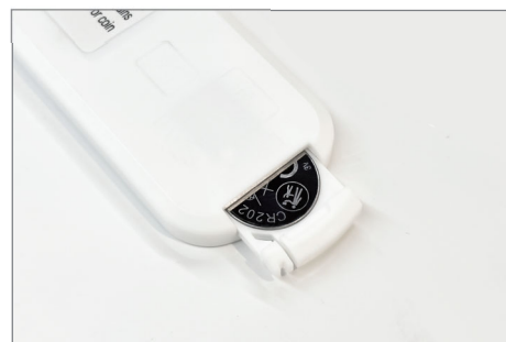
Install the Button-Cell Battery with the Correct Polarity
