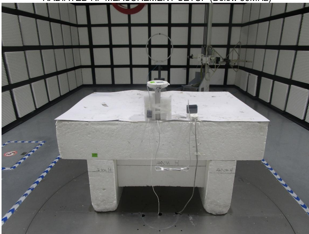
RADIATED RF MEASUREMENT SETUP (Below 30MHz)
