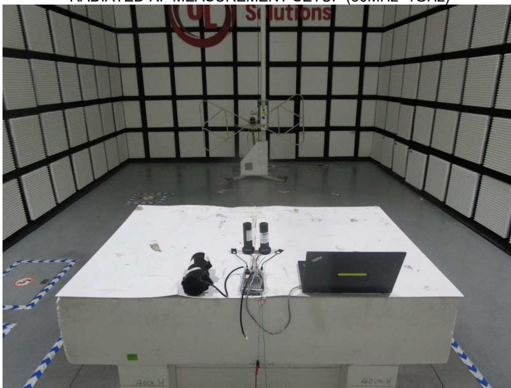
RADIATED RF MEASUREMENT SETUP (Below 30MHz)
