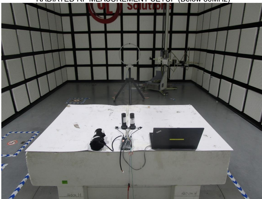
RADIATED RF MEASUREMENT SETUP (Below 30MHz)
