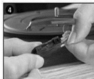
Remove the audio-line from the cartridge.
