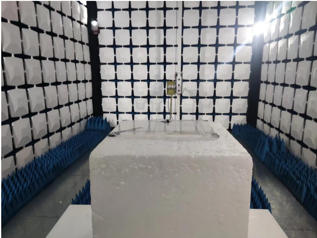
Above 1GHz for radiated emission test setup
