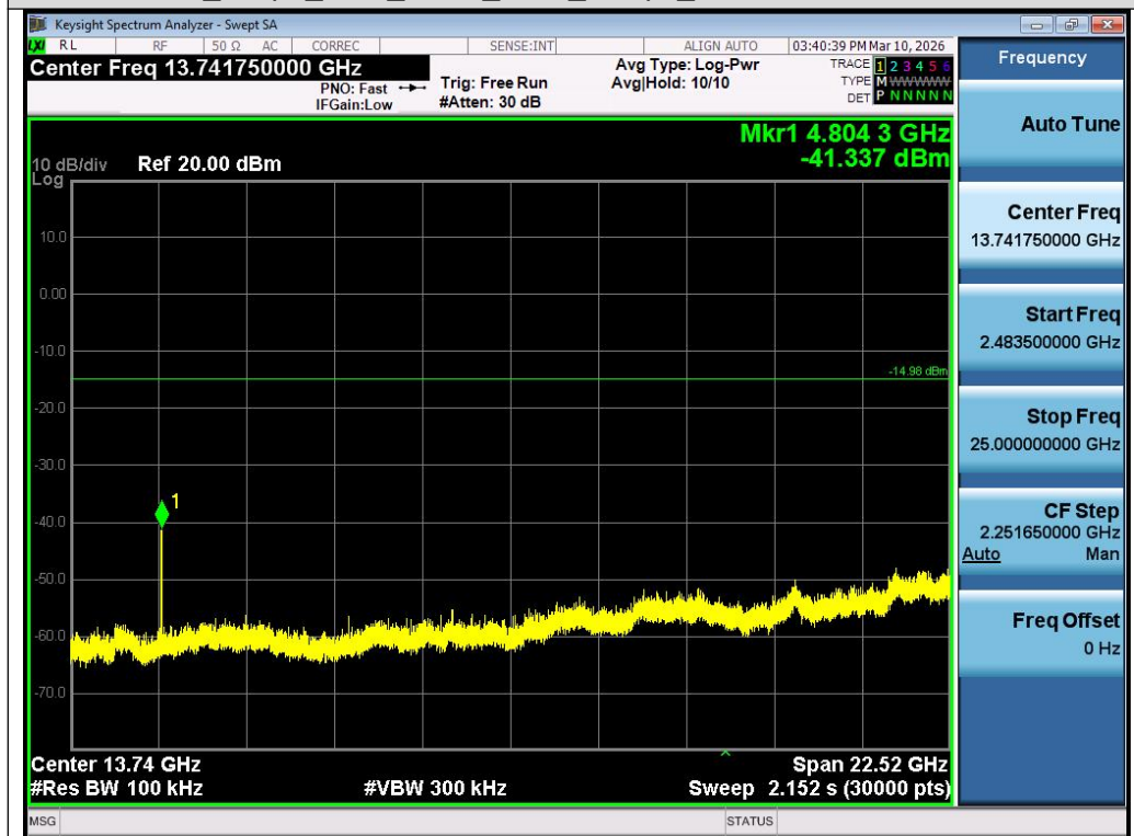
Test_Graph_EDR_ANT1_2402_2Mbps_Higher Band Emissions
