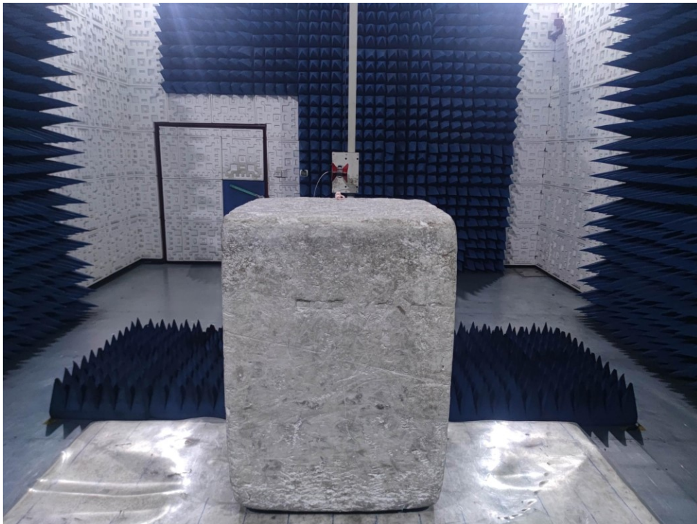
RADIATED EMISSION TEST SETUP ABOVE 1GHz
