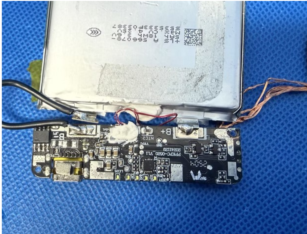
INTERNAL VIEW OF EUT (FIGURE 10) _With lithium battery protection circuitry
