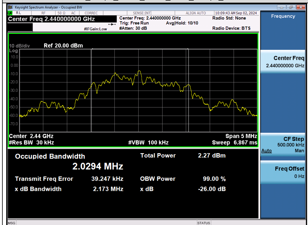
Test_Graph_LE2M_ANT1_2440_2Mbps_OBW
