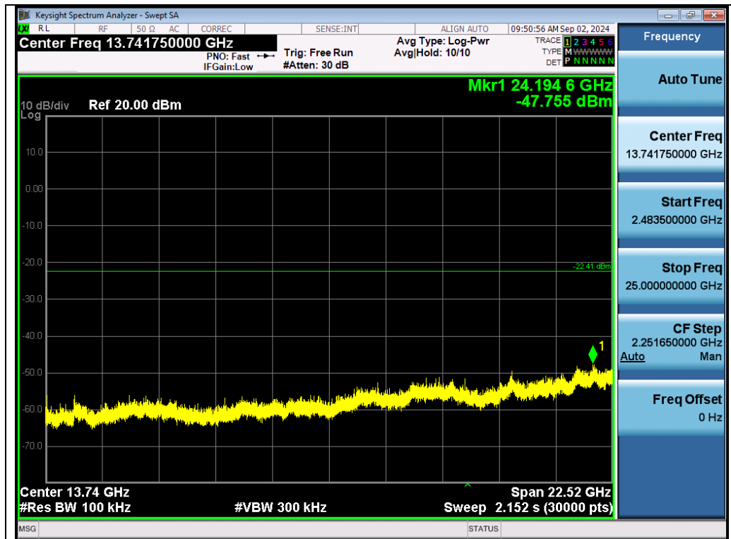
Test_Graph_LE1M_ANT1_2402_1Mbps_Higher Band Emissions
