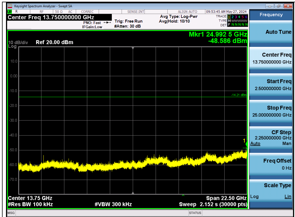
Test_Graph_LE1M_ANT1_2480_1Mbps_Higher Band Emissions
