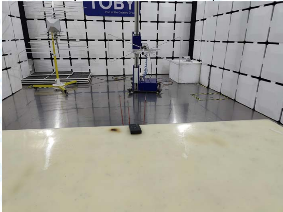
Photo of Setup for Radiated Emission (Below 1 GHz)
