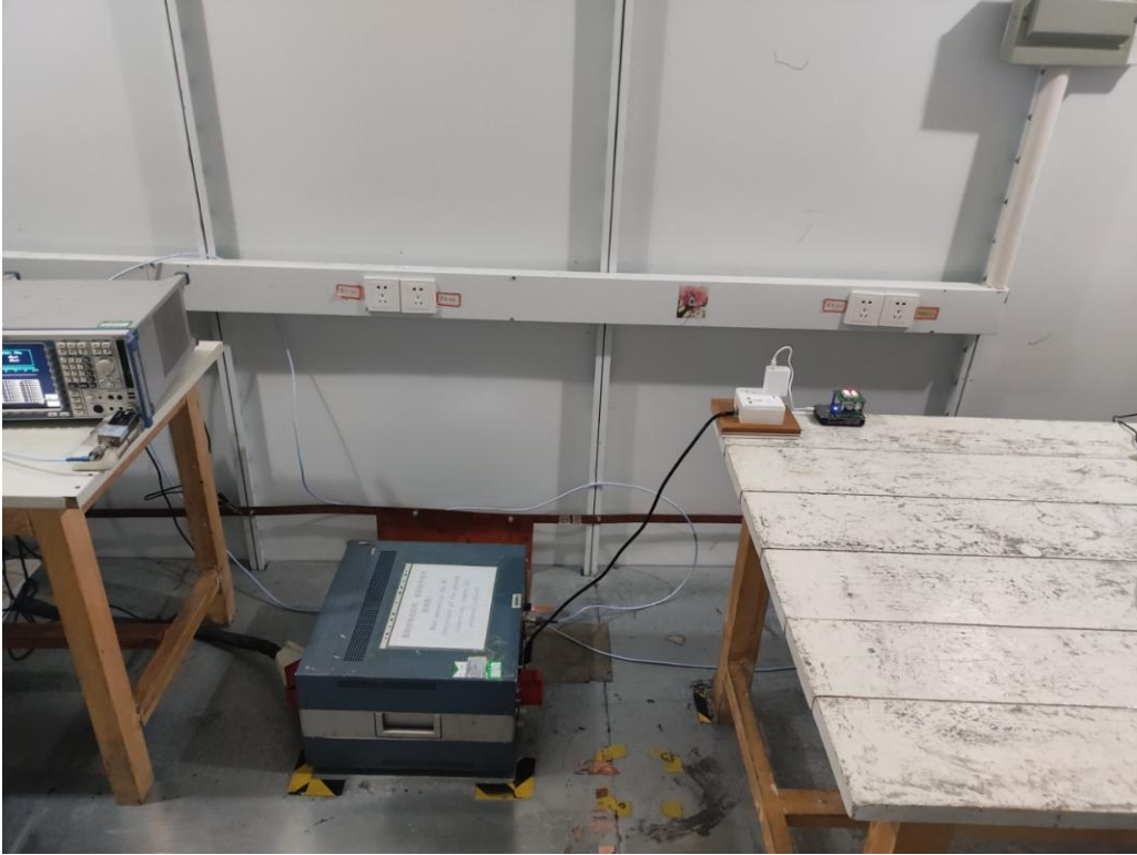
Photo of Conducted Emissions Measurement
