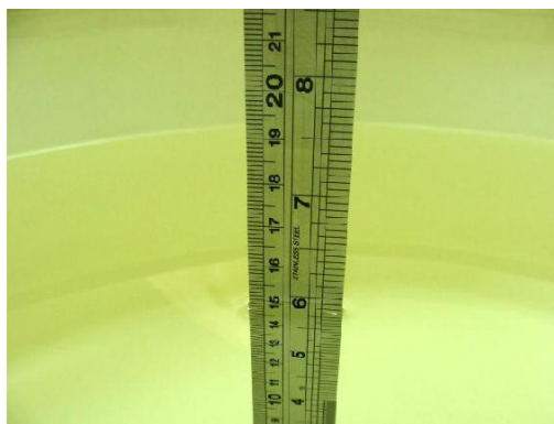
Fig 7.2 Photo of Liquid Height for Body SAR
