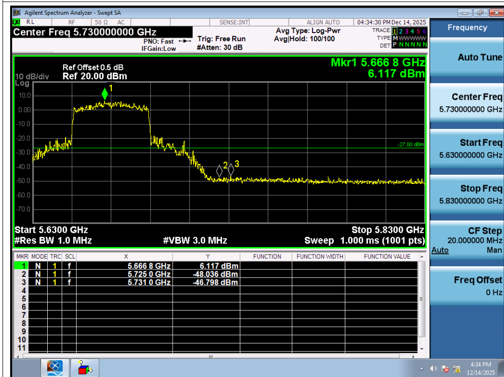
Band Edge NVNT ax40 5670MHz High Ant1
