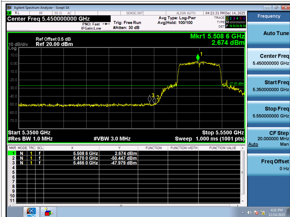
Band Edge NVNT n40 5670MHz High Ant1
