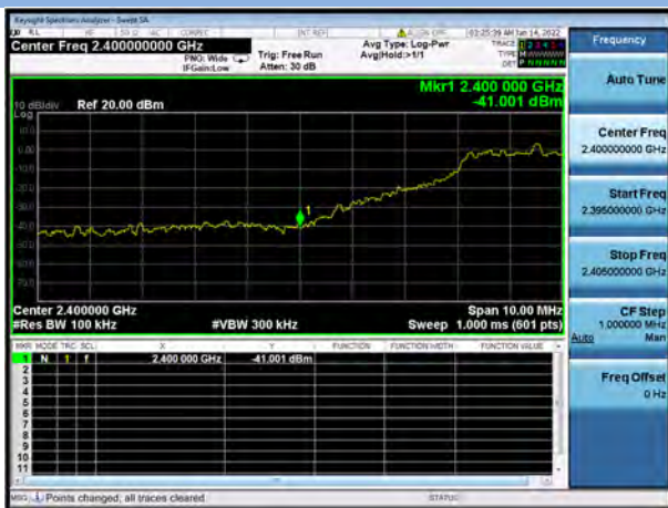
802.11n-20 MHz CHANNEL 1, Reference level
