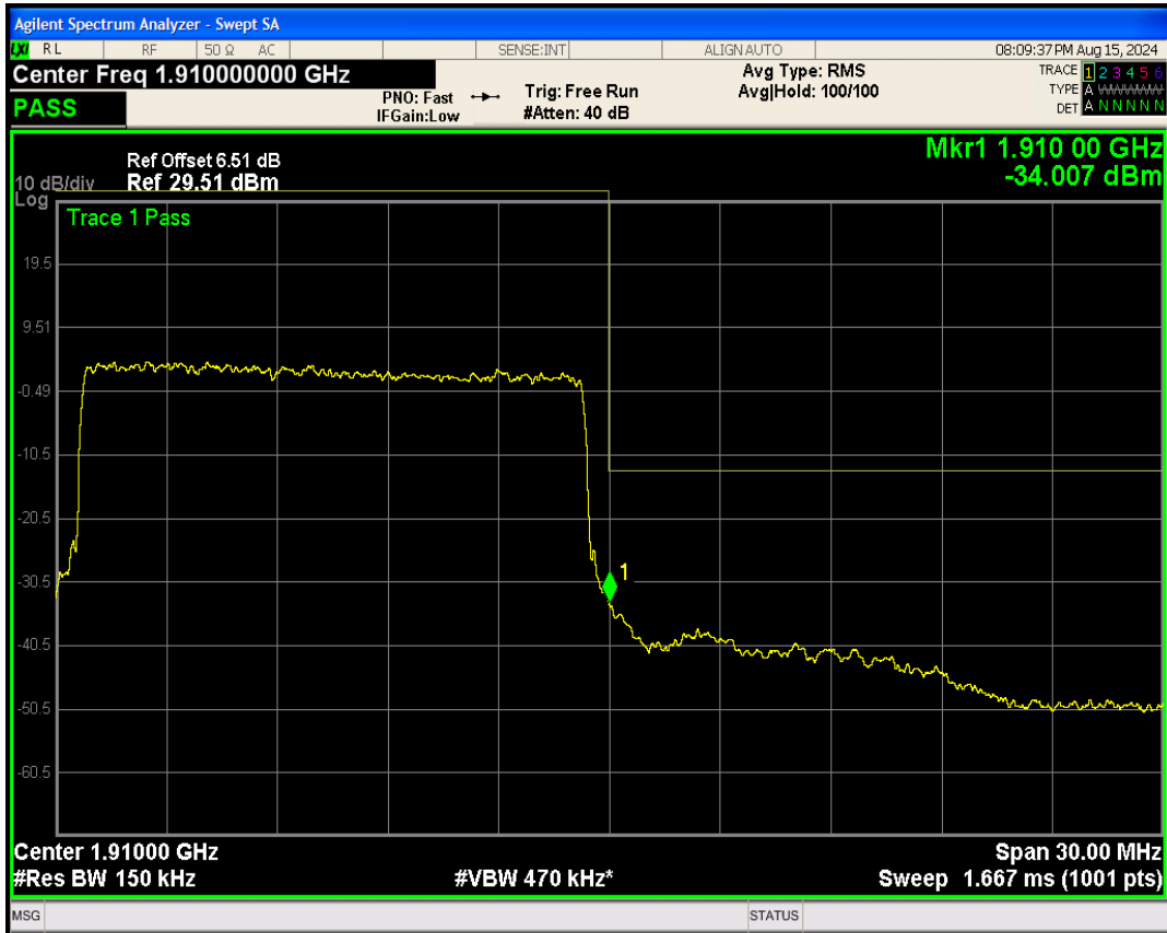
Band2 16QAM BW=15MHz Channel=19125 RB Size=75 Position=#0
