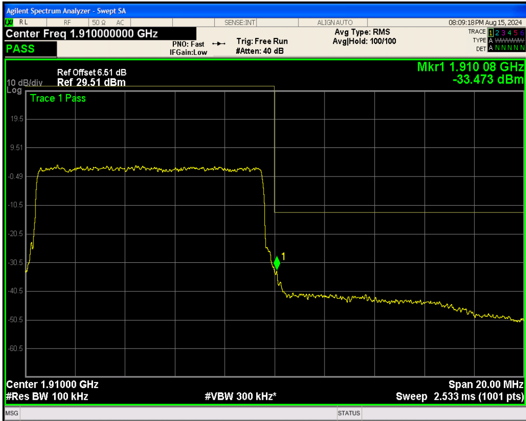
Band2 16QAM BW=10MHz Channel=19150 RB Size=50 Position=#0
