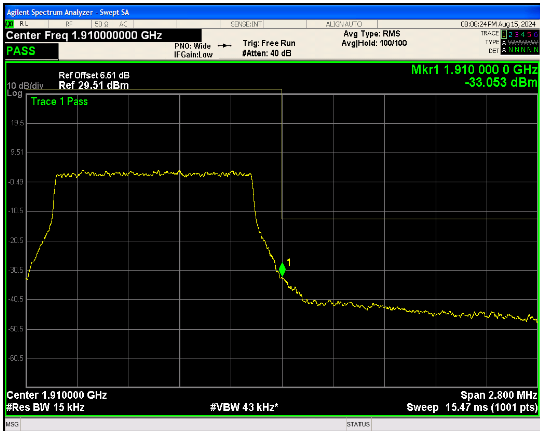
Band2 QPSK BW=3MHz Channel=18615 RB Size=15 Position=#0
