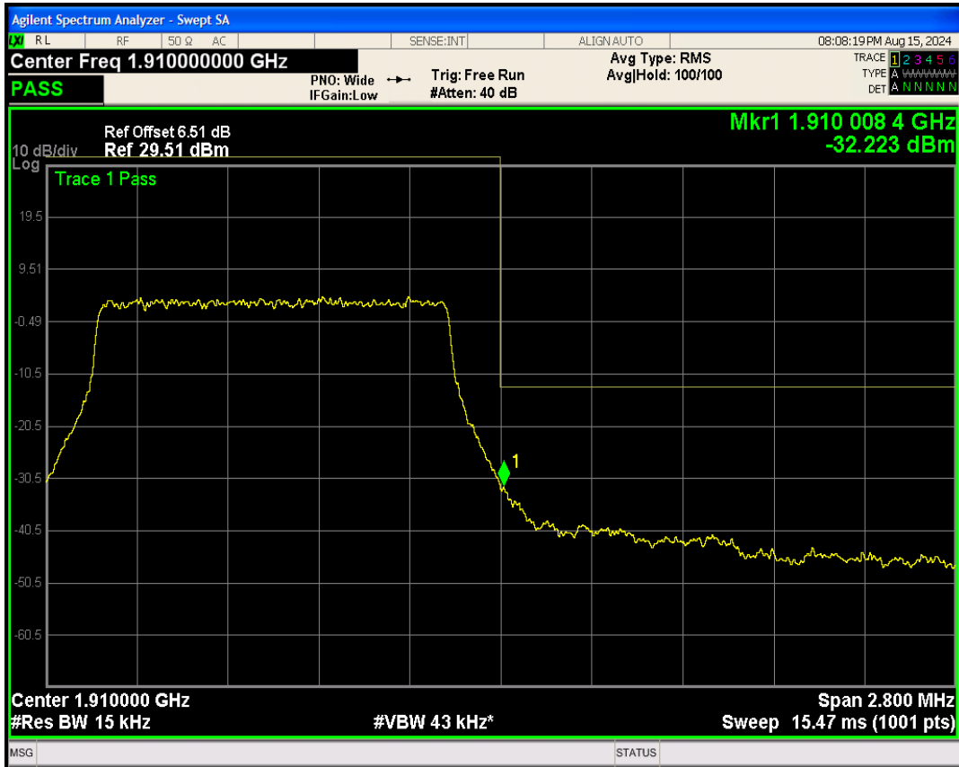
Band2 16QAM BW=1.4MHz Channel=19193 RB Size=6 Position=#0
