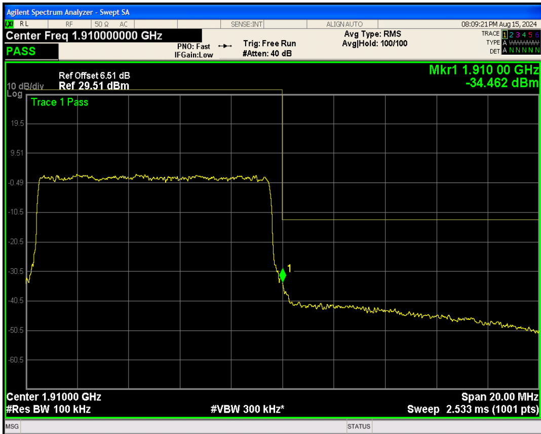
Band2 QPSK BW=15MHz Channel=18675 RB Size=75 Position=#0
