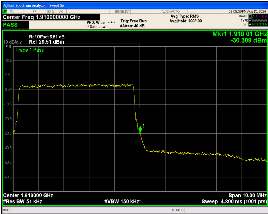
Band2 16QAM BW=5MHz Channel=19175 RB Size=25 Position=#0
