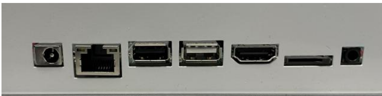
12V DC IN RJ45 OTG-USB USB HDMI OUT TF CARD EARPHONE
