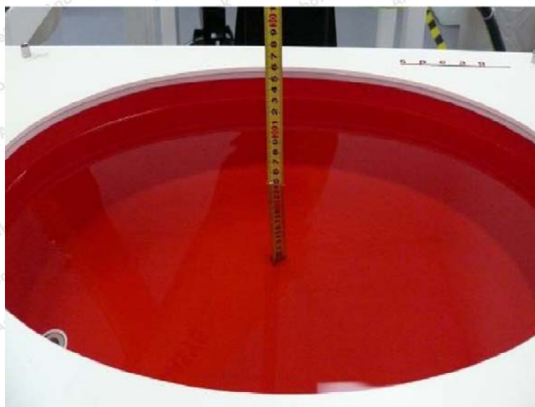
Photograph of the depth in the Body Phantom (450MHz, 15.4cm)
