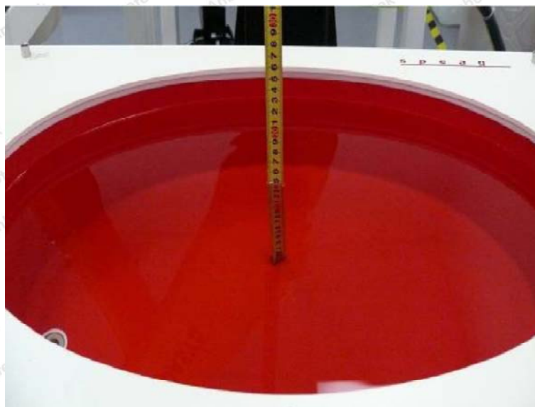
Photograph of the depth in the Head Phantom (450MHz, 15.3cm)
